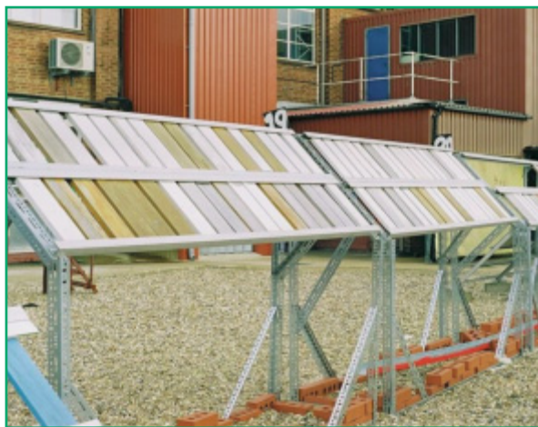
Natural exposure of experimental coatings as part of the test programme. (Courtesy of Anthony Buxton of the Paint Research Association)
