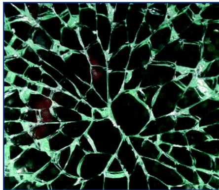
Butterfly-shaped failure in glass indicating nickel sulfide as the cause.
