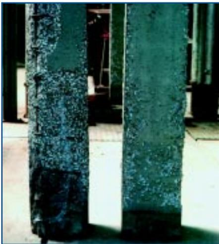
C85 reinforced concrete columns after fire testing. The column on the left has no polypropylene fibres; the other column has 3kg of fibres per kg of concrete.
