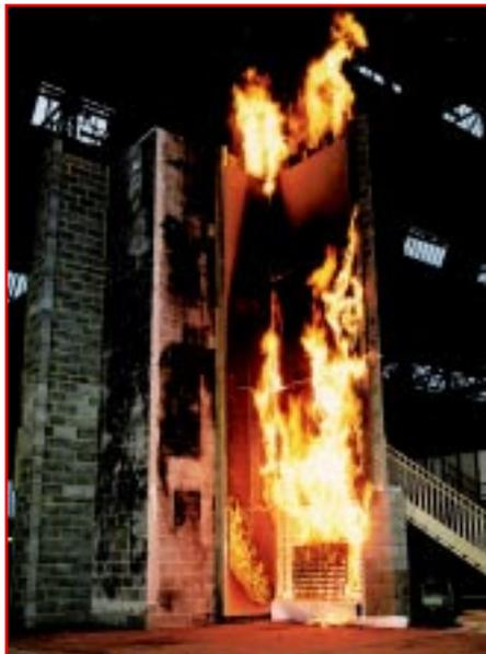
Cladding fire test at BRE Cardington
