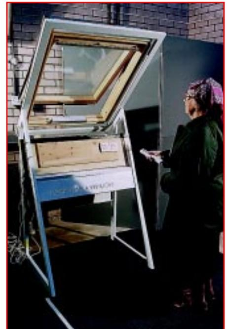
(Right) Roof window system used in laboratory tests: top and horizontal pivot, chain operator works in top hung outward opening mode, remote control or key pad activators, linked in system to timber.
