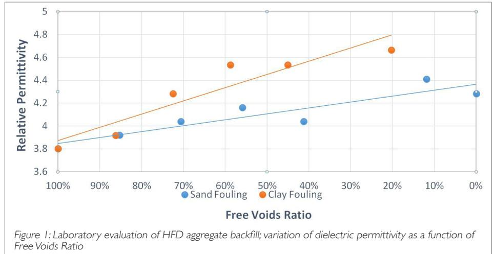
Figure 1: Laboratory evaluation of HFD aggregate backfill; variation of dielectric permittivity as a function of Free Voids Ratio
