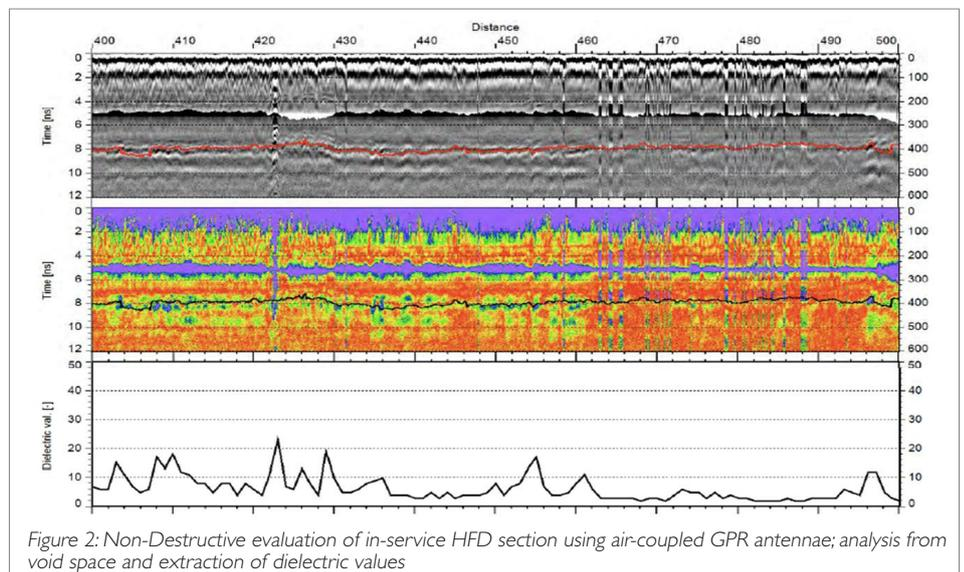
Figure 2: Non-Destructive evaluation of in-service HFD section using air-coupled GPR antennae; analysis from void space and extraction of dielectric values
